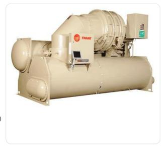
compressor is about 2950rpm, with low speed and few running parts. Cold discharge can be as low as 10% without surge.
