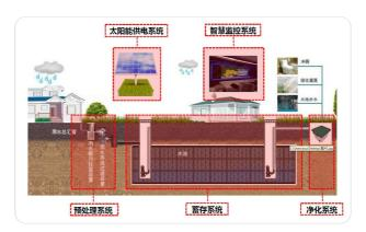
independently developed by Zhongke Shiwo Ecological Technology Jiangsu Co., Ltd. The rainwater recovery system adopts a smart monitoring system and is incorporated into the Huiyun management platform to record the collection, usage and supplementary water capacity of rainwater in real time. Solar photovoltaic power generation is used to provide system operating energy.
