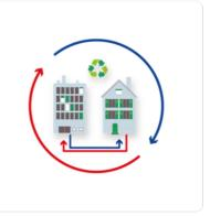
The key factor in the 5GDHC approach is the optimal reuse of return flows at different spatial and temporal scales. Energy storage is used to manage the temporal imbalance between supply and demand within the system on a daily, but also seasonal basis.
