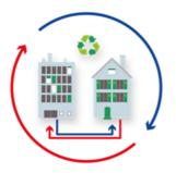
The first principle of 5GDHC is to avoid wasting energy in the system. A 5th generation grid differs from other heat and cooling grids in its ability to exchange energy with other connected consumers/customers: it is a circular thermal network. The network is designed as a closed loop reusing energy as much as possible: the heated buildings provide cold to the system, while the cooled buildings transmit their excess heat to the network.
