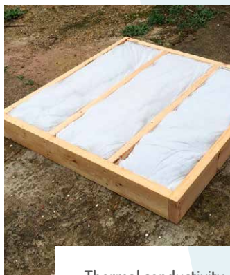
100 to 150 mm-thick wall panel
