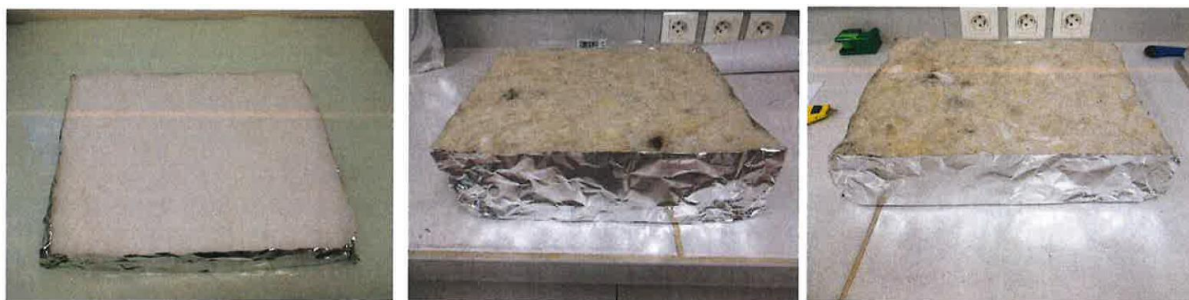
Figure 4 : Test specimens (Prototypes 1, 2 and 3) after cutting and sealing
