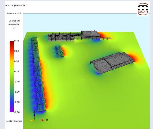
$$\frac{\partial}{\partial x_i} \left[ \rho \overline{u}_i k - \left( \frac{\mu_T}{\sigma_k} \right) \frac{\partial k}{\partial x_i} \right] = \mu_T \left( \frac{\partial \overline{u}_i}{\partial x_j} + \frac{\partial \overline{u}_j}{\partial x_i} \right) \frac{\partial \overline{u}_j}{\partial x_j} - C_\mu \frac{k^{3/2}}{L_T} \text{ and } \mu_t = \rho k^{1/2} L_T$$
