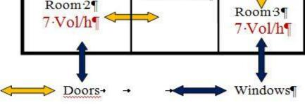
Ex : doors area=windows area =  $2 \text{ m}^2 =>$  Internal pressure losses reduce ACH by 20%
