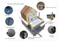
Services connect the house with land. Insulated and flexible pipes run along the side of the house, within the wet dock, to pump wastewater into a treatment tank set in the ground.
