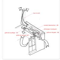
The originality of the solution lies in the fact that, unlike most natural ventilation strategies which are based on sweeping between an air intake in the lower part and an outlet in the upper part, we implement ventilation paths supply and extraction so that these flows intersect, thus allowing the implementation of heat
