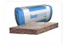
Thanks to the structure of its entangled glass fibers and the immobile air trapped in its pores, the glass wool has a high insulating power with a minimum of material. This makes it a lightweight insulating product with thermal performance ranging from 0.030 W / (m.K) to 0.040 W / (m.K), certified by ACERMI.
