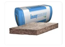
Thanks to the structure of its entangled glass fibers and the immobile air trapped in its pores, the glass wool has a high insulating power with a minimum of material. This makes it a lightweight insulating product with thermal performance ranging from 0.030 W / (m.K) to 0.040 W / (m.K), certified by ACERMI.
