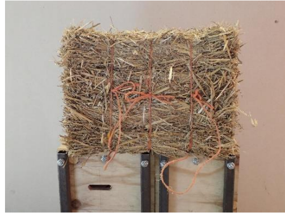
Figure 1: Optimised straw bales in an OSB frame (left); optimised straw bale (right)
