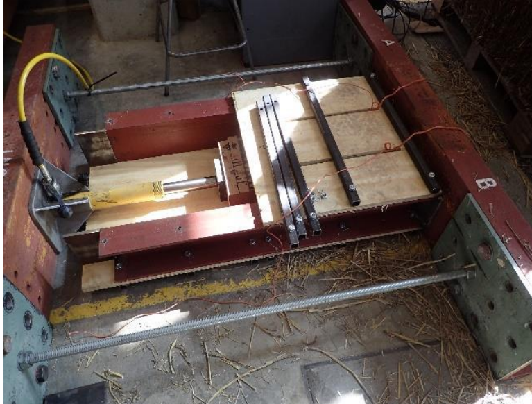
Figure 3: Hydraulic press built and used by the University of Bath to produce prototypes
