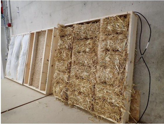
Figure 1: Optimised straw bales in an OSB frame (left); optimised straw bale (right)
