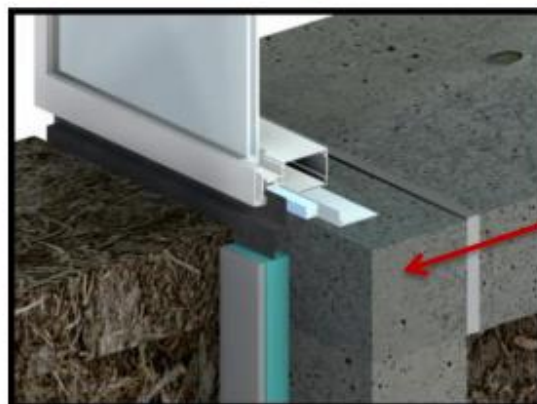
Perimeter heat loss for curtain-wall at-grade by varying U-values
