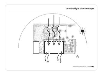
favor of trellises in order to promote natural ventilation, the shutters are rehabilitated for solar protection, air blowers are put in place to ensure cooling throughout. of the year.
