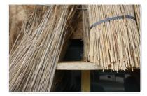
Insulation Stubble on wooden and OSB cleats fixed on concrete façade: The peripheral activity rooms have been requalified using vertical thatch. Concurrently assuming the roles of insulation and finishing, this unprocessed natural product has been implemented for the first time in France in renovation applied on concrete facade. It offers a thermal mantle and assumes its share of acoustics.
