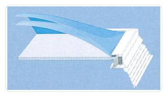
not have good thermal insulation values. A booster frame was installed to better encapsulate the outlet and its concrete base for the insulation of the roof. In addition, the model we chose has an airgel plate which reduces the U value of the outfall. It also improves the distribution of light. Thanks to that, the staircase enjoys good natural lighting.
