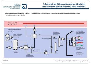
thermal systems on the roofs of their buildings. The quarter is located not far away from the cogeneration plant Adlershof. The BTB's modern cogeneration plant is powered by natural gas and feeds the heat, which is generated by 90% in cogeneration, into a network that goes far beyond Adlershof, which also supplies the newly connected residential district.
