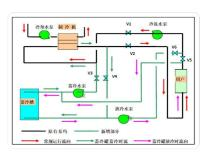
Water storage technology refers to that when the power load is low at night, the cold amount produced by the electric refrigerator is stored in the form of cold water. At the peak time during the day, do not open or partly open the refrigerator to make full use of the cold amount stored at night for air conditioning so as to achieve the purpose of power peak load shifting.
